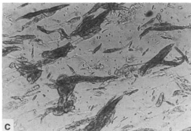
Figure 5 Hot-stage photomicrographs ( \times 260 ) of the partially drawn fibres: (a) PP/Vectra A900 (100/10); (b) PP/Vectra B950 (100/10) and; (c) PP/Rodrun LC3000 (100/10)
